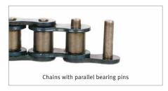
For breaking chains with parallel pins it is necessary to grind off the rivet heads on one side of the chain. Afterwards the outer link is pressed out as above.
