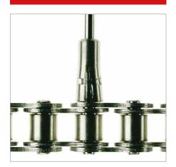
Insert the adapter into the jaws ① and break it by closing the tool. If necessary, repeat the action after 45° rotation. Once the adapter has been broken, remove the pin.
