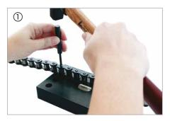
The outer link to be broken has to be placed over the holes in the riveting plate (D). The bearing pins are hammered flush with the outer plate and then driven through the chain with pin punch (B) whose diameter must be smaller than that of the bearing pin 1.
