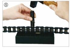
The newly fitted outer link then requires the bearing pin ends to be riveted. This is done with riveting punch (E) **5**.
