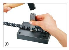
A new outer link plate is fitted using fetching-up punch (C) 4. With parallel bearing pin chain it is possible to over fit the outer link plate on the bearing pins. It is necessary to check that the joint remains free and easily moveble after fitting.
