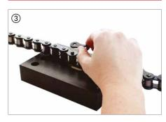
The procedure used is common to both shouldered and parallel bearing pin chains. The new riveting link connects the two inner links. This connecting link is supported by an insert in riveting plate (D) ③.
